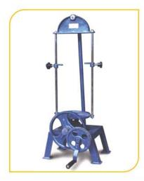
This is a bench type model, which is portable, sturdy and convenient for bench mounting. The side-to-side rocking motion carrier can accommodate 7 sieves.
