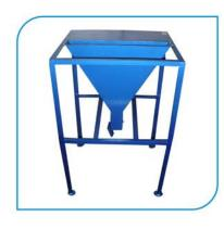
This instrument is used to assess the fluidity and segregation resistance of Self Compacting Concrete.
